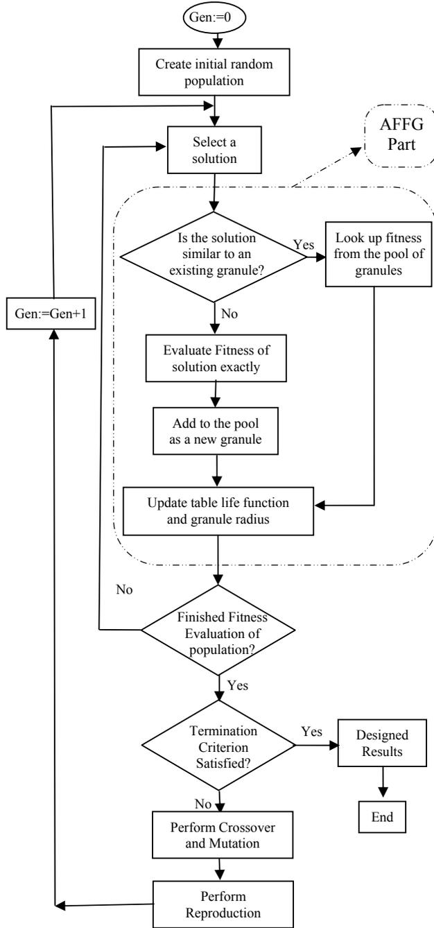
Figure 1. Flowchart of the Purposed AFG Algorithm
