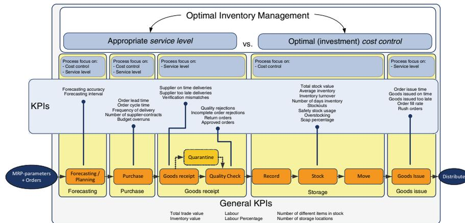
**Fig. 4.** The designed Inventory Performance Measurement Framework showing the tension between providing a high, appropriate service level versus optimal cost control in terms of KPIs for the different sub-processes in IM and the overall IM process
